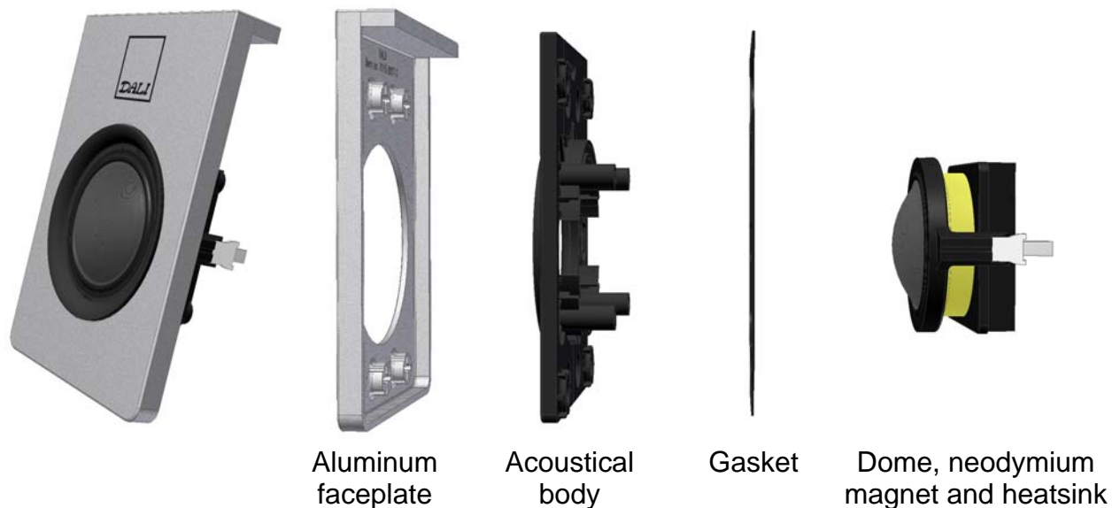
Figure 3, Exploded view of 28mm neodymium tweeter for LEKTOR® 1.
